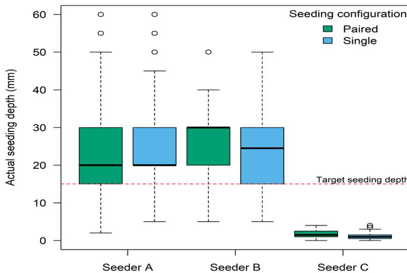
Figure 2: Actual seeding depth versus the target seeding depth of 15 mm for three seeder machines used in the 2018 and/or 2019 seasons. Seeder A and B are both DBS seeders but owned by different growers. Seeder C is a John Deere Airhoe drill. For each boxplot, the bold line indicates the median seeding depth, the coloured box indicates 50% of the data range, whiskers represent 95% of data range and dots represent outliers.
